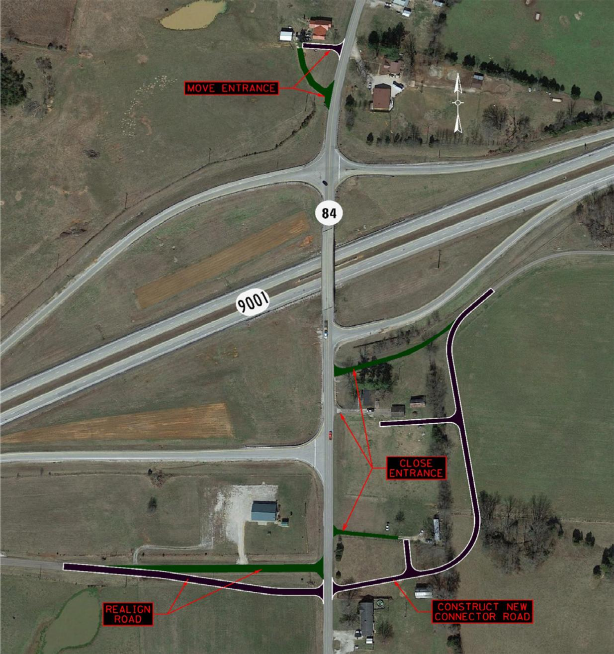
Figure 28: Exit 136, US 31W Bypass Control of Access Improvement
